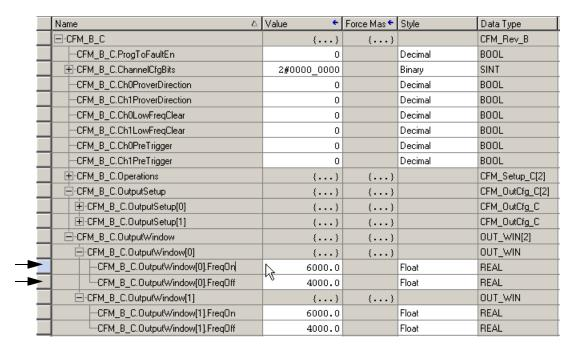
**3.** In the Value column of the CFM\_B\_C.OutputWindow data tags, enter the desired the On and Off frequency limits.
