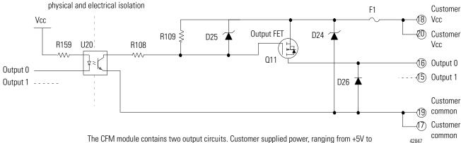
The CFM module contains two output circuits. Customer supplied power, ranging from +5V to +31.2V DC, is connected internally (through terminals #18 and 20) to the power output transistors. When an output is turned on, current flows into the source, out of the drain, through the load connected to the ground of the customer supply (customer return). Diode D26 protects the power output transistor Q11 from damage due to inductive loads.
