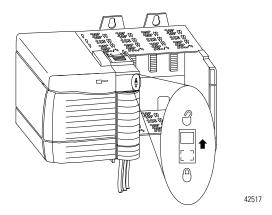
**2.** Open the RTB door and pull the RTB off the module, as shown in Figure 5.2.
