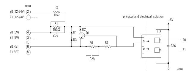
To turn on a gate circuit, you must source current through the input resistors sufficient to turn on the opto-isolator in the circuit. If no connection is made to the pair of gate terminals, no current will flow through the photodiode of the opto-isolator and that gate will be OFF (the corresponding input status indicator is OFF).
