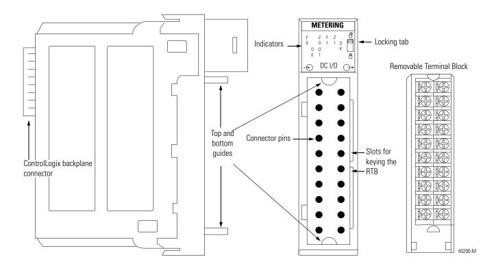
**ControlLogix backplane connector** - The backplane connector interface for the ControlLogix system connects the module to the ControlLogix backplane.
