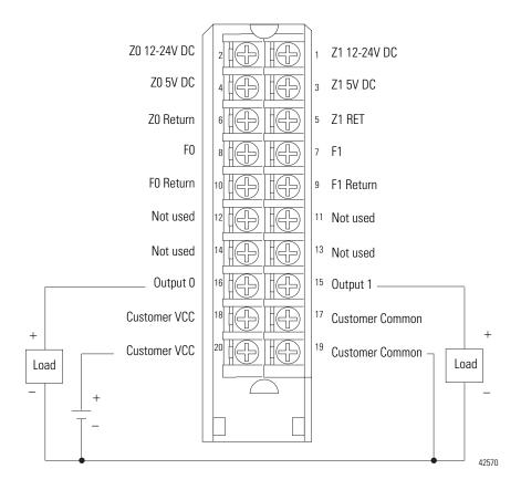
NOTE: If separate power sources are used, do not exceed the specified isolation voltage.
