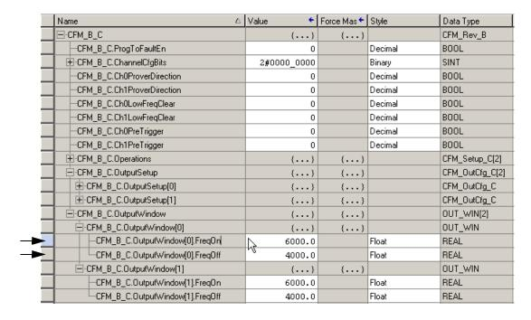
**3.** In the Value column of CFM\_B\_C.OutputWindow FreqOn and FreqOff data tags, enter the desired On and Off frequency limits.
