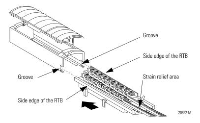
2. Slide the RTB into the housing until it snaps into place.
