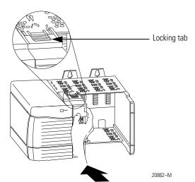
2. Slide the module into the chassis until the module locking tabs click.
