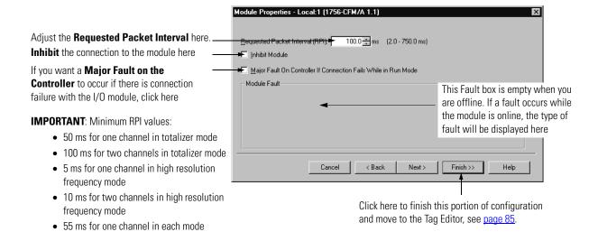
After you are finished with the screen above, you must access the module tags, via the Tag Editor, to make additional configuration changes, see <u>page 85</u>.
