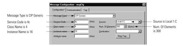
This table contains information that must be entered on the configuration screen to perform the example CFM module service:
