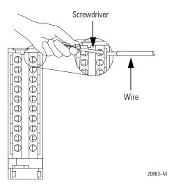
**3.** Insert the wire into the open terminal and remove the screwdriver.
