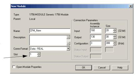
Enter the slot number that matches the location of the 1756-CFM module in your ControlLogix chassis.
