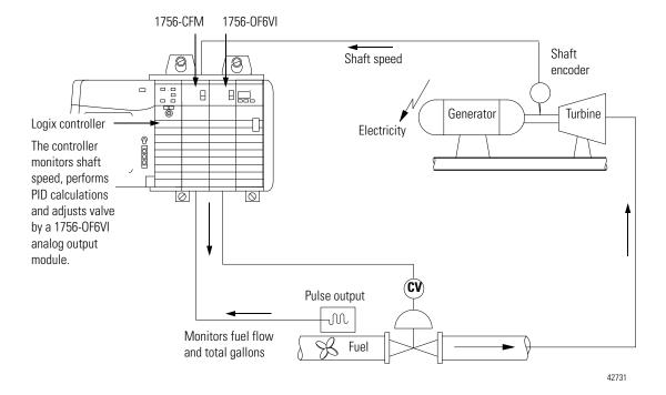
For a detailed explanation of how the CFM module works with other portions of a ControlLogix control system, see Chapter 2, Configurable Flowmeter Operation in the ControlLogix System.
